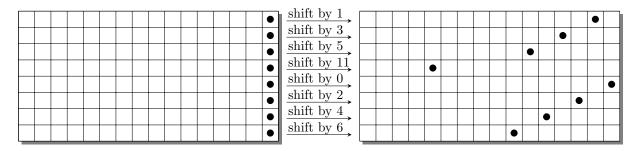
Figure 2: The ShiftBytesWide<sub>Q</sub> transformation.
